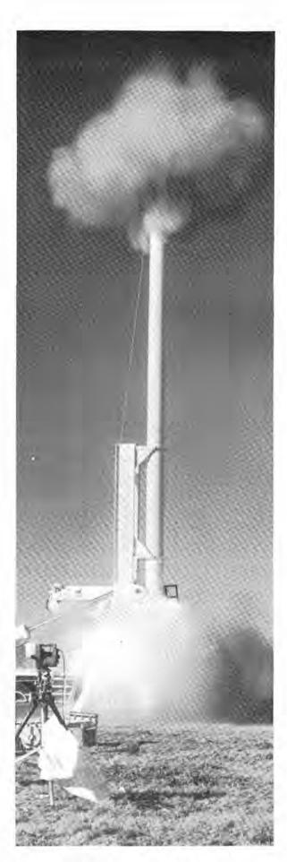
NEW DOWN-FIRING GUN recently underwent a series of test firings near Edgewood. The gun is used to fire projectiles into the ground as part of the Labs' continuing terradynamics program.
